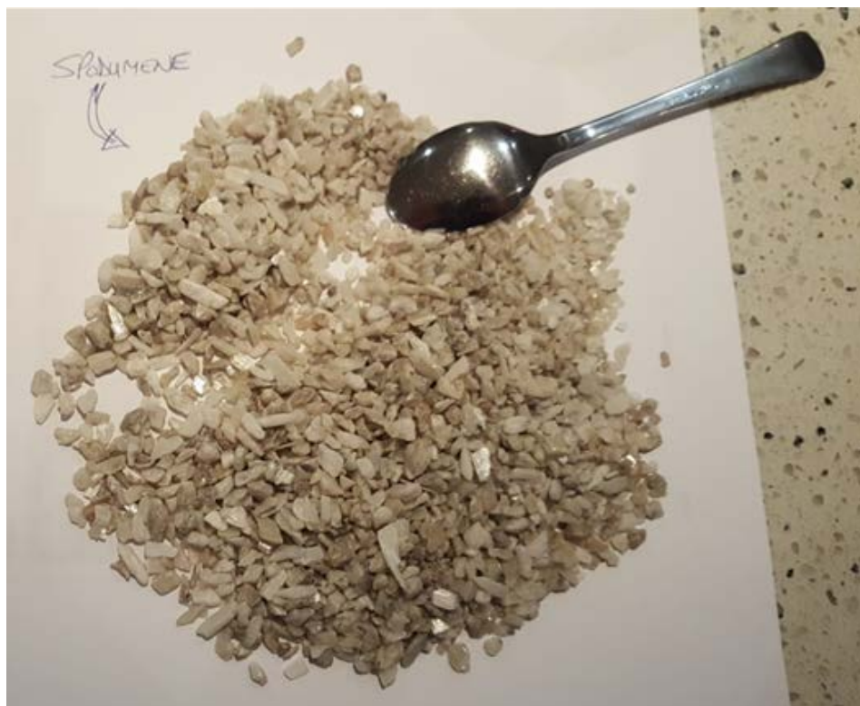
Figure 1.8 Picture of Spodumene as an SC6 Concentrate
