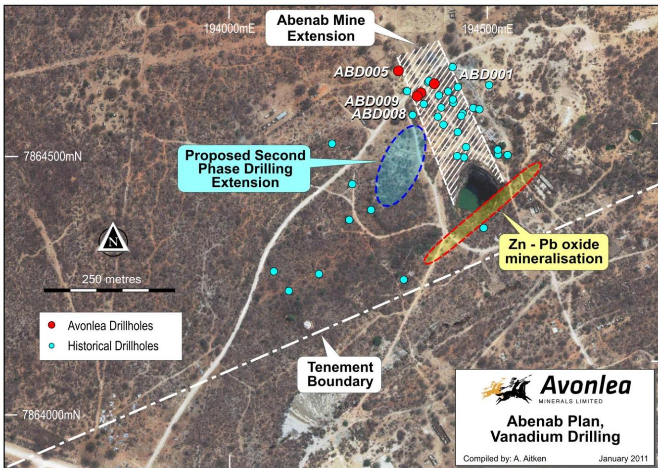
Figure 1: Plan view of the Abenab prospect, including current and historical drill hole locations.
